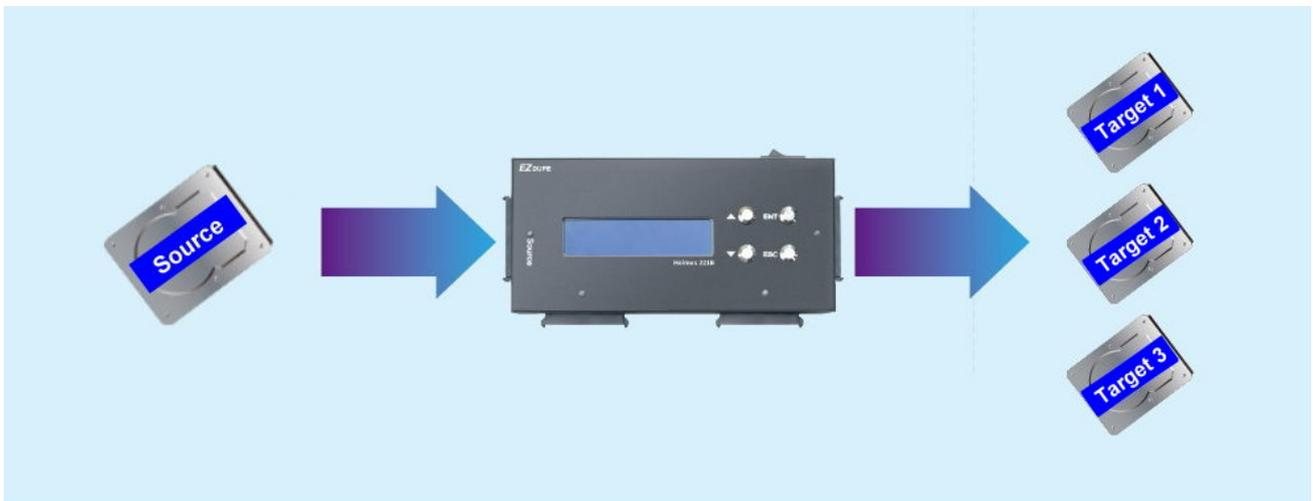
**Disk to File** Images the source disk to a file and stores in a large image disc. The different image files can be stored in a large image disc in sequence. Images HDD 1 then HDD2 and then HDD 3.
