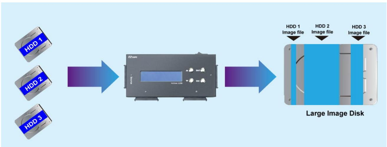
**File to Disk** Restores image file from a large image disc to target disks. Users can choose one
